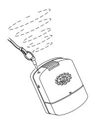
To activate both Mugger Stopper Plus alarm and strobe light, simply pull out pin on top of unit.
